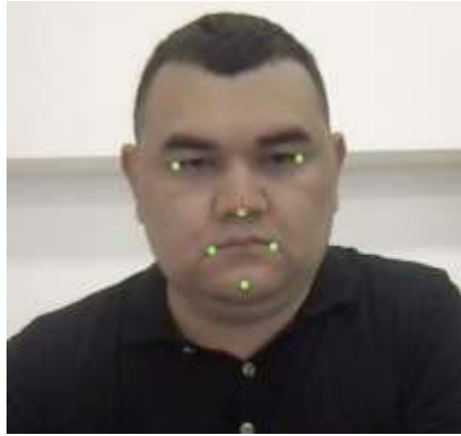
Fig. 1. Visualizing the output of the landmark detection algorithm.
